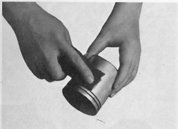
Fig. 3-37 Polishing piston surface
