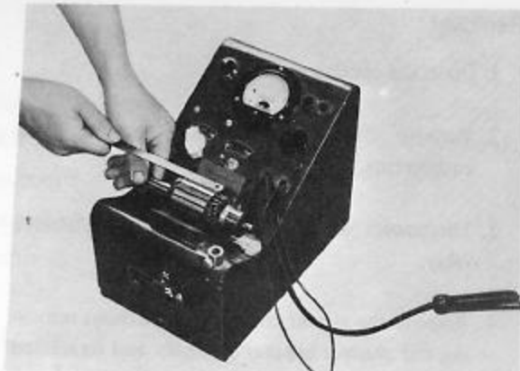
Fig. 10-10 Checking armature for short circuit
