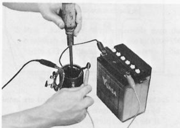
Fig. 10-13 Checking field coil by exciting it
