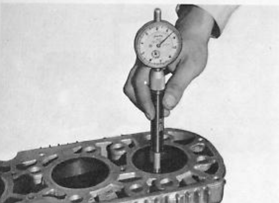
Fig. 3-30 Measuring cylinder bore for wear
