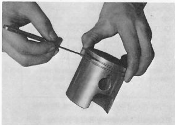
Fig. 3-39 Measuring piston ring side clearance
