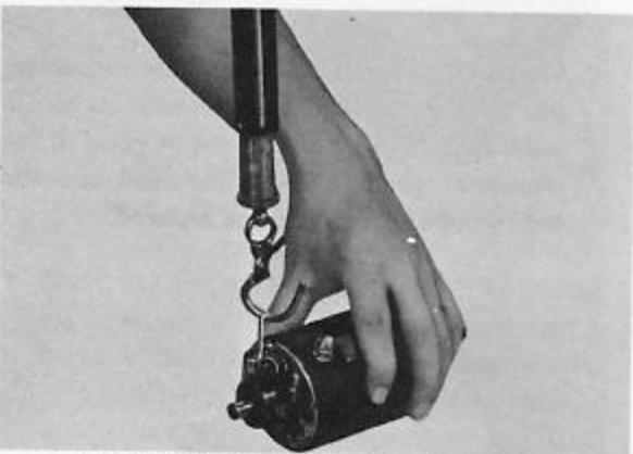
Fig. 10-18 Checking brush spring tension
