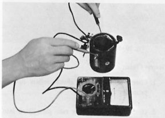
Fig. 10-16 Checking field coil for ground
