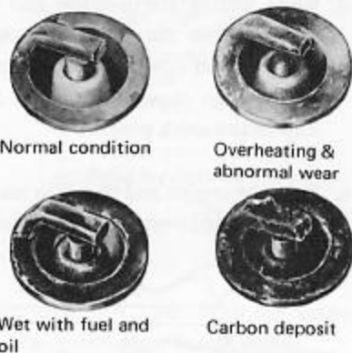
Fig. 10-40 Condition of spark plug
